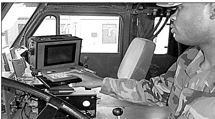
Soldiers used the Movement Tracking System—a mounted, rugged, GPS-equipped computer—to track many of the supply trucks used in Iraq.
